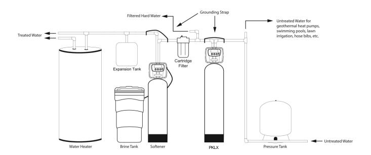
FIGURE 1: Typical Installation
